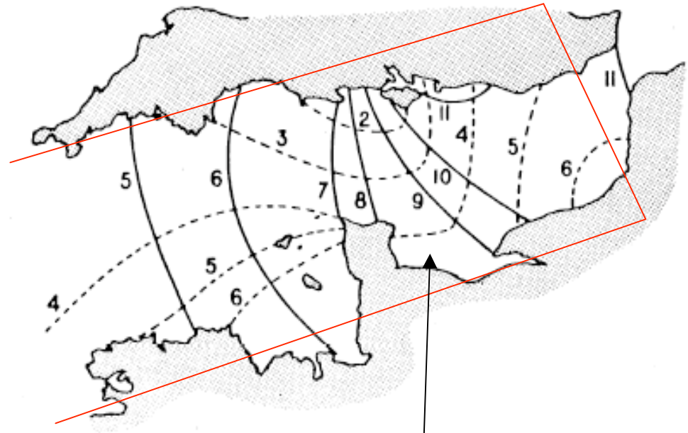
Fig. 10.5. Co-tidal lines (solid) with time in lunar hours, and co-range lines (dotted) with the English Channel. [From Proudman (1953, p. 262); after Doodson and Corkan (1931).]
