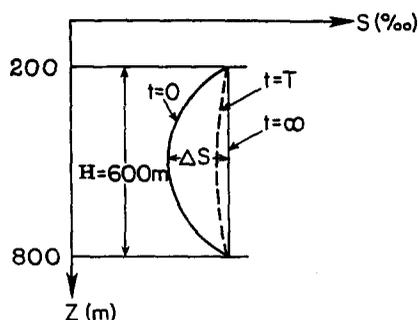
Fig. 10. Model configuration used to estimate the effective vertical eddy diffusivity required for the salinity–depth curve to relax from its initial profile at  $t=0$  to the nearly straight profile at  $t=T$ .
