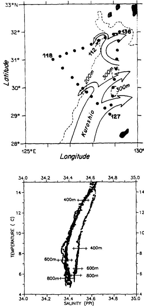
Fig. 9. Schematic of vertically averaged absolute geostrophic current field in triangle region during January 1986 taken from CHEN *et al.* (1992) (upper panel) and *T/S* curves for CTD Stas 127–136 along eastern transect (lower panel). Also shown on the upper panel are 200 and 300 m isobaths taken from the East China Sea Bathymetry Chart (provided by Second National Institute of Oceanography, P. R. China).
