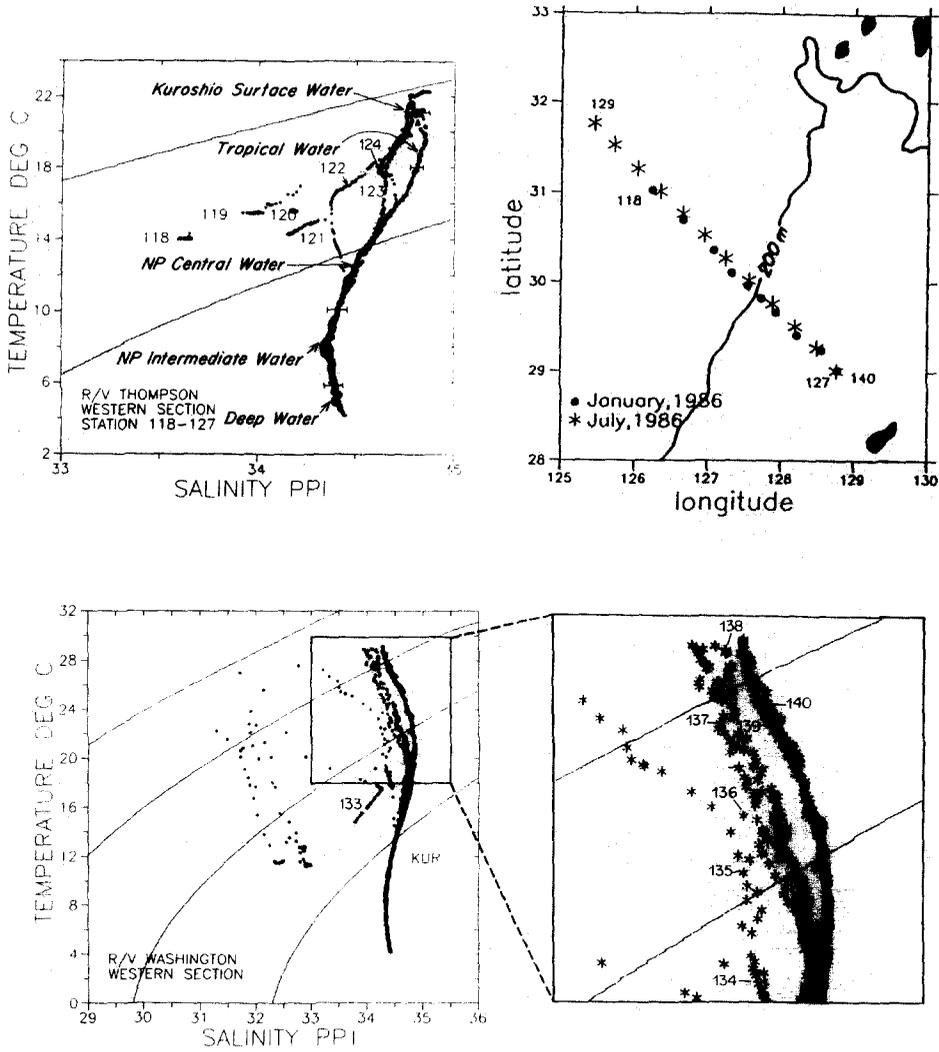
Fig. 8. *T/S* curves for CTD stations on the western transect for January (upper) and July (lower) 1986. The station locations are shown in the upper right panel and an enlargement of the July *T/S* curve is shown in the lower right panel.
