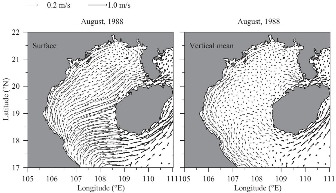
**Figure 15.** Maps of Global-FVCOM-computed August (left) monthly averaged surface and (right) vertically averaged) current vectors in the Gulf of Tonkin for the homogenous case with only wind forcing (Ex1).
