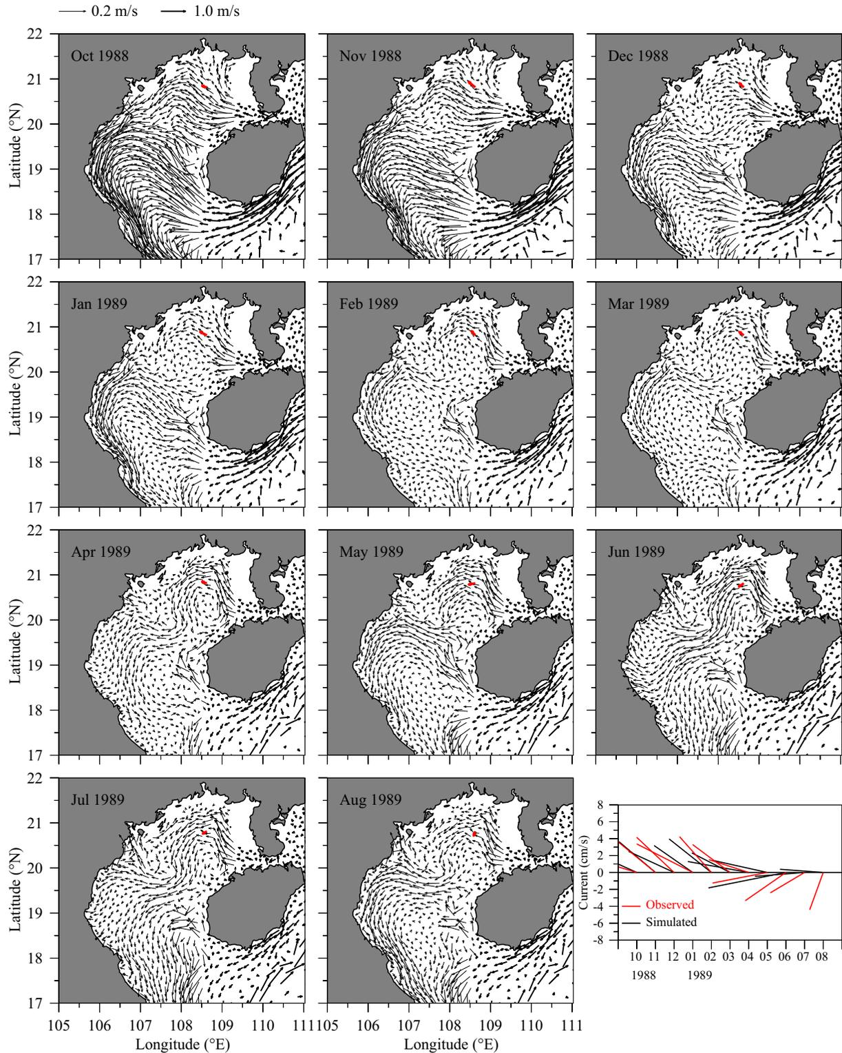
**Figure 13.** Maps of Global-FVCOM-computed monthly averaged current vectors at 10 m depth in the Gulf of Tonkin for the period October 1988 to August 1989. Monthly averaged current vectors observed at 10 m depth at site A are superposed in these figures (red vectors). The comparison of the 10 m model-computed and observed monthly mean vector currents at site A is shown in the bottom right plot.
