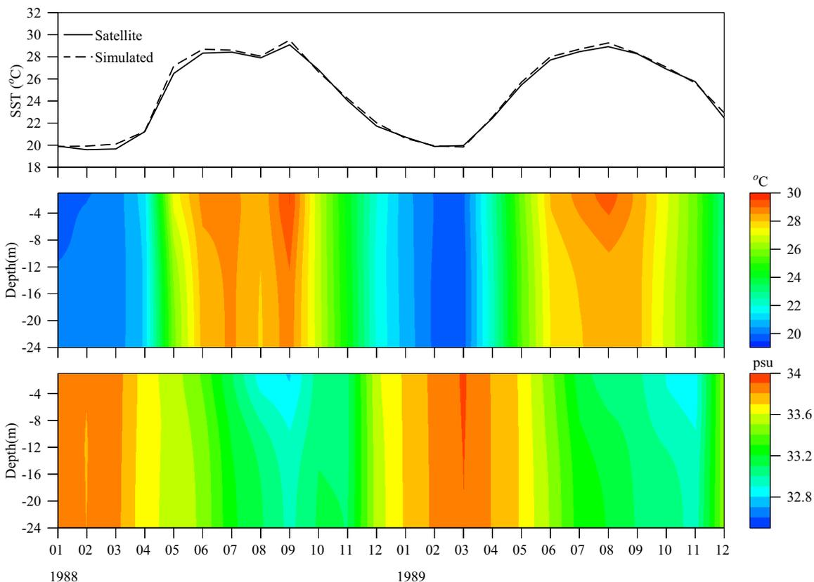
**Figure 9.** Time series of (top) the satellite-derived sea surface temperature (SST) and (middle) the Global-FVCOM-calculated temperature and (bottom) salinity at site A from January 1988 to December 1989.
