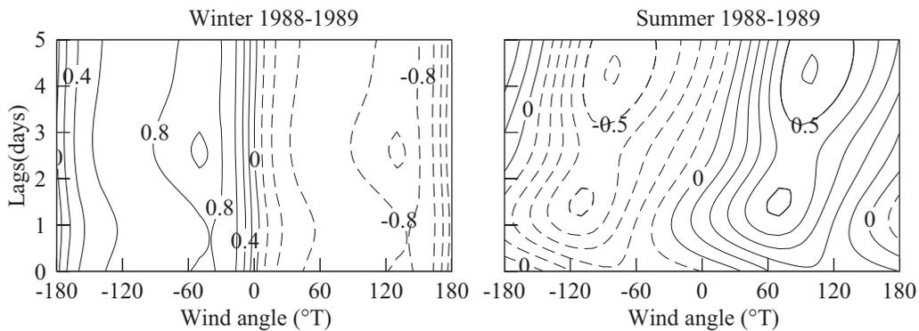
**Figure 11.** Correlations between observed subtidal currents at 10 m depth and surface wind velocity at 10 m height for the winter and summer seasons of 1988–1989. Analysis was done by projecting subtidal currents to the northwest direction. The critical value was 0.22 for a 95% confidence level.
