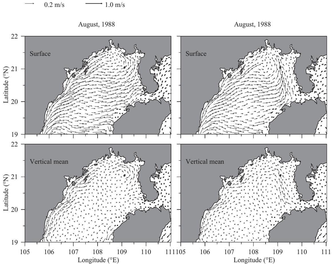
**Figure 17.** Maps of Global-FVCOM-computed August (top) monthly averaged surface and (bottom) vertically averaged current vectors in the northern Gulf of Tonkin for the stratified cases (left) with only wind forcing and (right) with wind plus tidal forcing.
